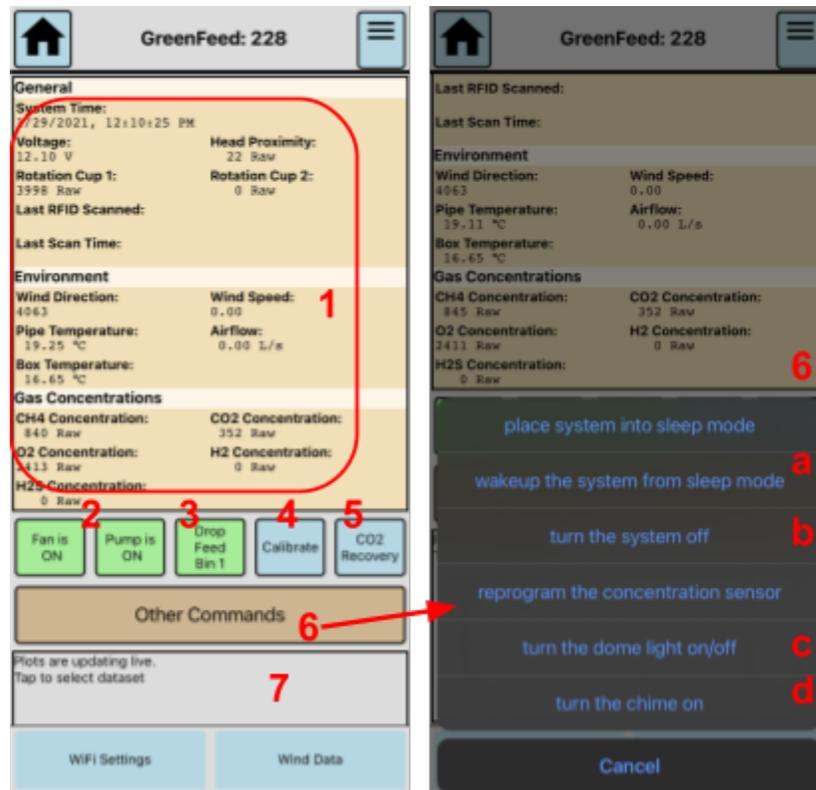
Figure 9) Viewing and Controlling a SimpleScan System from ControlFeed
